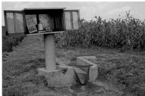
Figure 7.2 H-flume attached to a Stilling well and connected to a Drum-type Recorder for measuring runoff (Pathak, P. et al., 1981)
